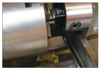
Photo 5. Lining the hole up with a drill shank.
