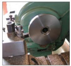
Photo 1. Turning the O.D. of the backplate true.
