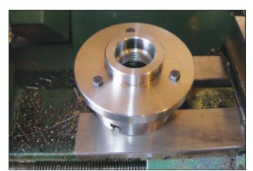
Photo 10. The backplate bolted to the chuck.
