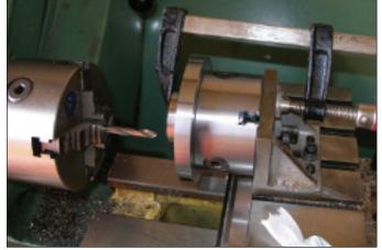
Photo 7. The backplate is clamped to the chuck.
