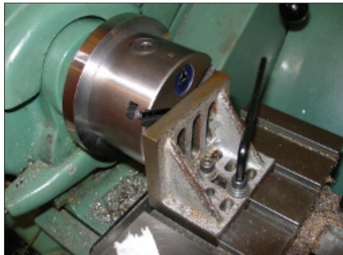
**Photo 3.** Setting the angle plate parallel to the chuck face.
