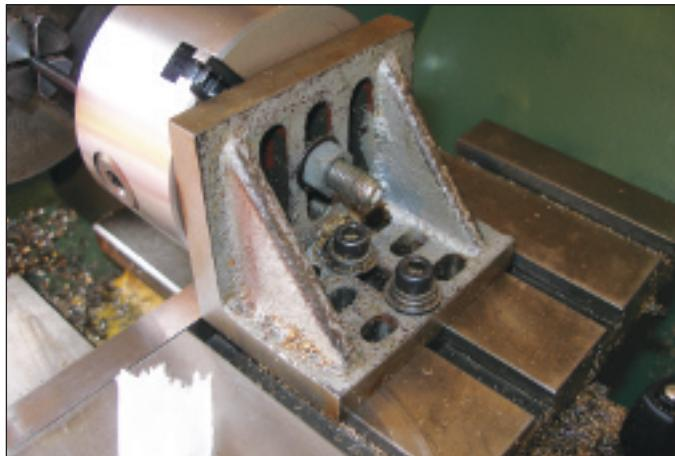
*Photo 6. The chuck is bolted to the angle plate by a bolt through the centre.*
