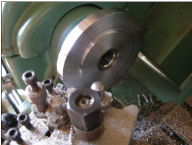
**Photo 2.** Chamfering the backplate after turning the chuck register.
