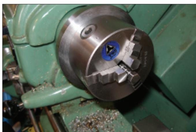
*Photo 11. The assembled chuck on the lathe.*
