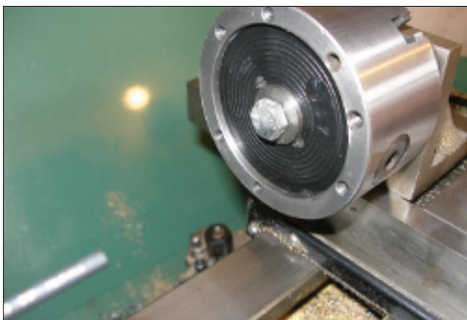
**Photo 4.** The chuck mounted on the angle plate.
