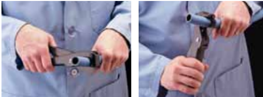
The rotating/rocking technique produces fast easy cuts.
